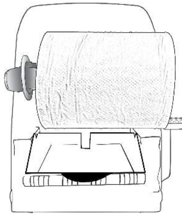
Load the roll with the paper tail at the back onto the left hand spindle
