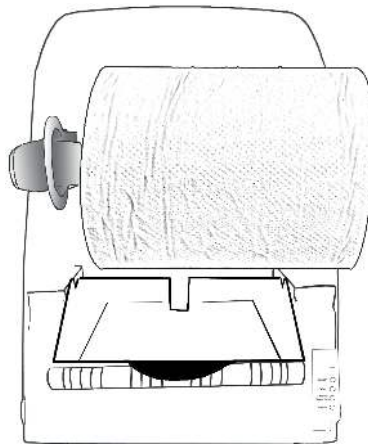
Load the roll with the paper tail at the back onto the left hand spindle
